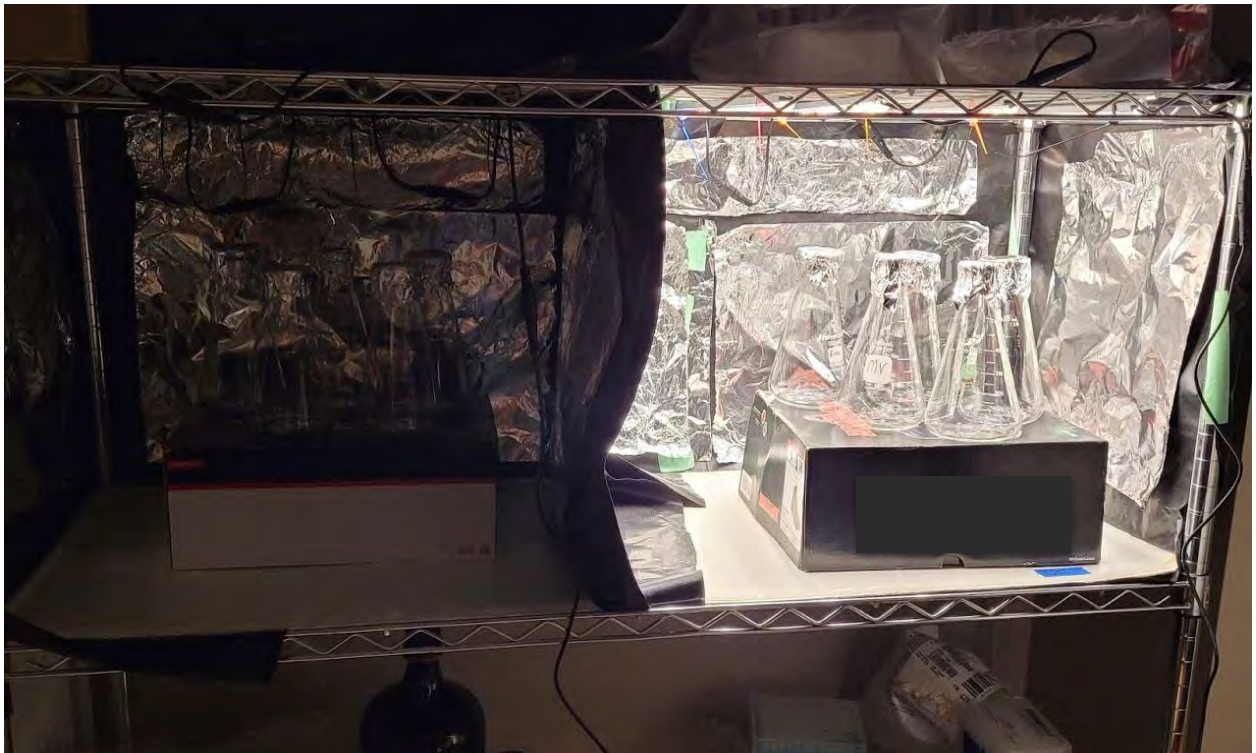
Figure 3. Culture set up with two chambers, separated by black plastic material, set to an alternating light cycle. Flasks elevated on boxes to achieve light intensity in Bigelow's recommended range (40 -120 \mu Einstein/s)
